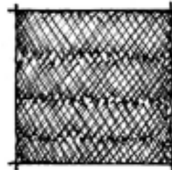
Cross Hatching (Continuous Lines)
